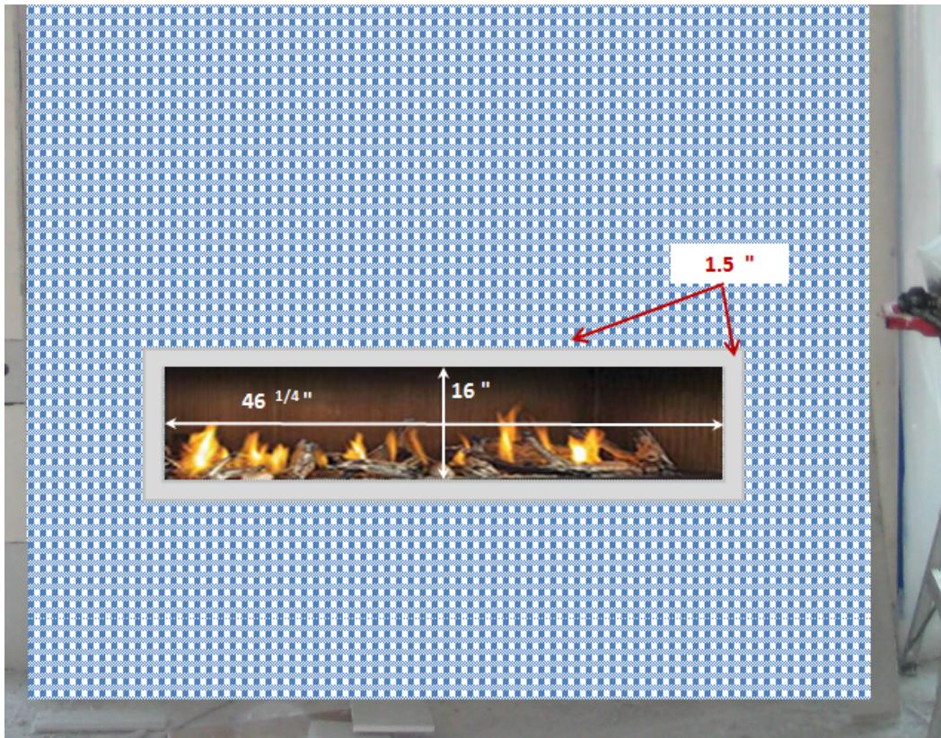
4. Once the tiles are installed, the surface of the tiles should be flush with the surface of the 1.5" metal surround
